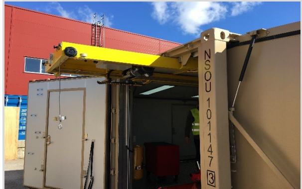
WORKSHOP WITH INTEGRATED EXTRACTABLE CRANE
